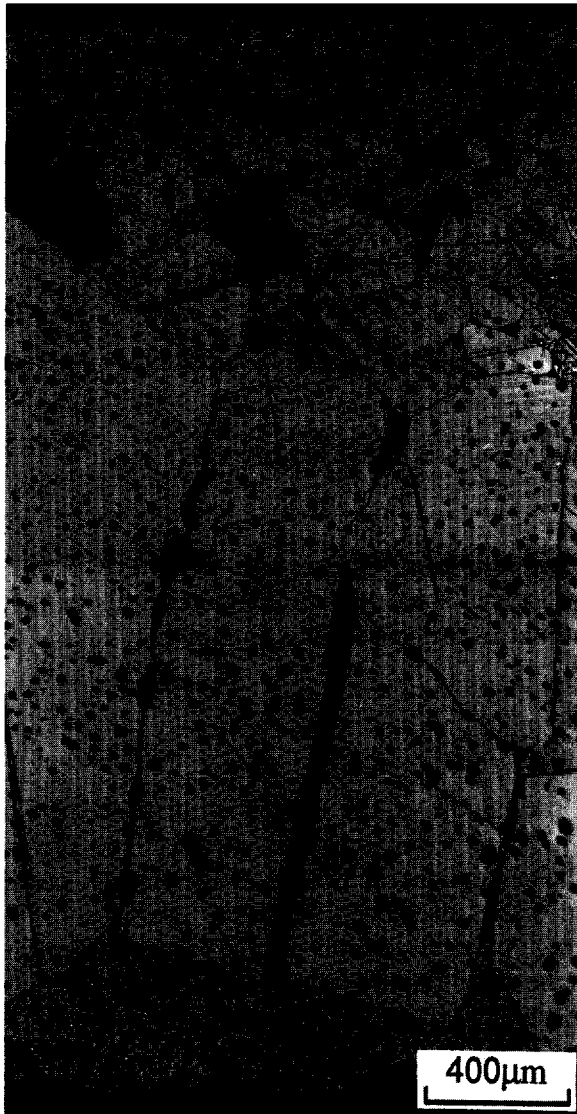
Fig. 1. Microstructure of the \text{BaTiO}_3 specimen. The \text{SiO}_2 slurry was dropped on top of the green \text{BaTiO}_3 compact and then heat-treated at 1350^\circ\text{C} for 8 h (From Ref. 1).
